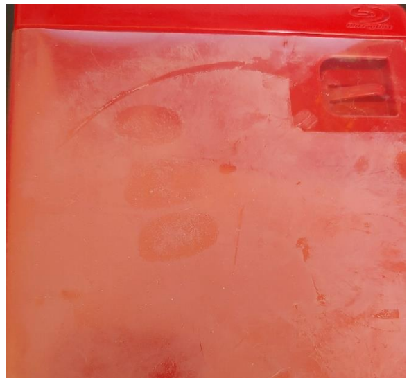
Superglue fumes react with prints on Blu-ray case after 3-4 hours.
