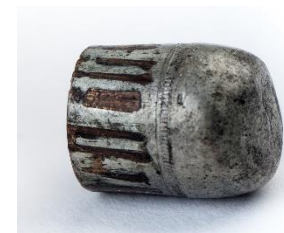
Bullet used in the St. Valentine's Day Massacre showing lands and grooves from rifling.
